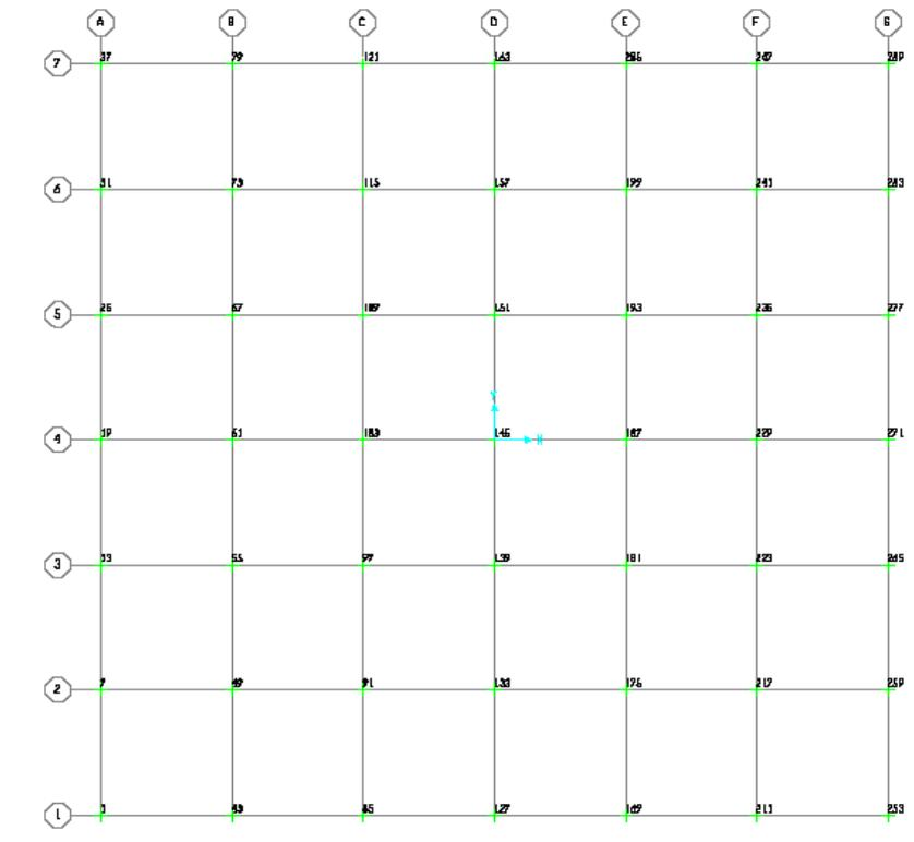
Fig.(5) Location of (Nllink)System for Building With Base Isolation.
