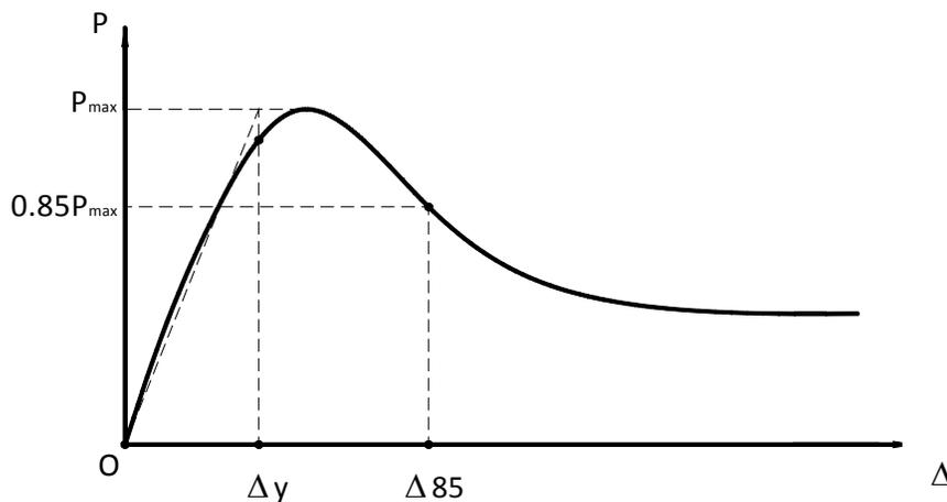
**Fig.(5) Determination of Column Displacement Ductility <sup>(10)</sup>.**
