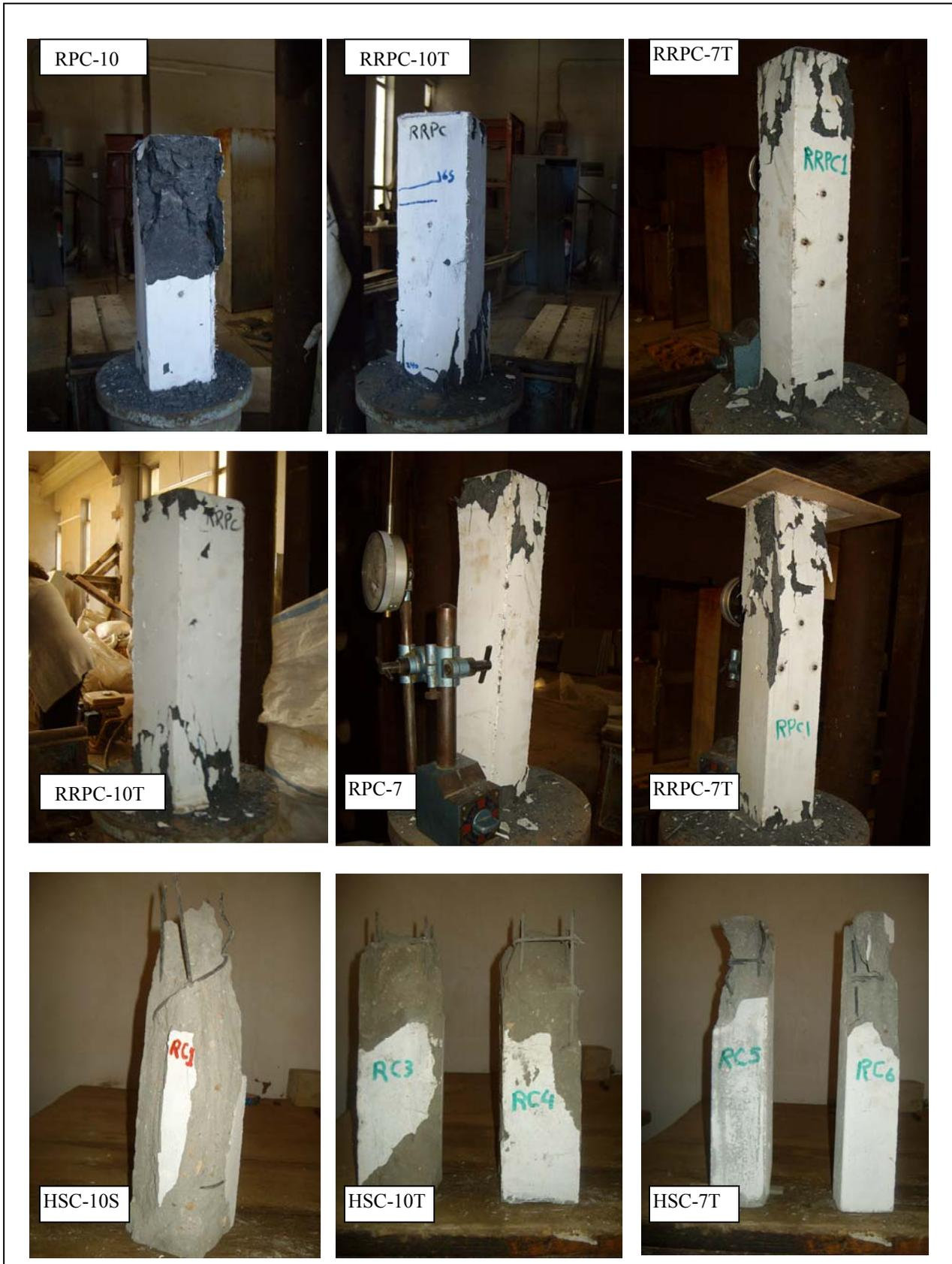
Fig.(3) Failure Mode of Column Specimens
